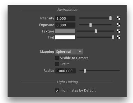
An environment light. The radius parameter controls the size of the sphere in the viewport.
