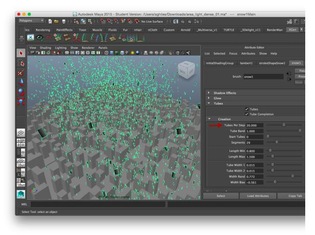
The test scene allows for procedural generation of floating area lights using the "Tubes Per Step" PaintEffects attribute.
