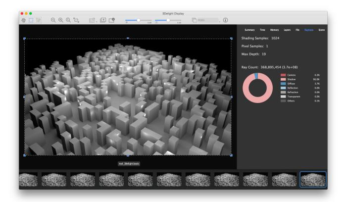
It is not uncommon for production scenes to rely heavily on geo area lights. In this test we will compare geo light **sampling technology** in 3Delight OSL, Ar nold and RenderMan/RIS. We will use a test with a geometric area light that is composed of a relatively large number of faces. The test, although limited, should allow us to find the convergence rate of each algorithm as well as general performance.
