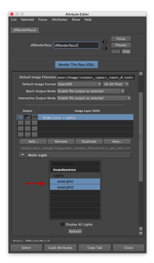
Select the two area lights to split the RGBA into two additional outputs (one for each area light)
