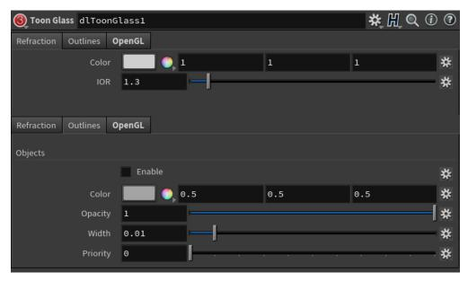
Toon Glass allows rendering a simple refractive material meant to be used in scenes using the Toon shader. It helps preserve the outlines and and particular shading of such surfaces when seen through a refraction. For this reason, it also has no *roughness* parameter, meaning the refraction is never blurred.
